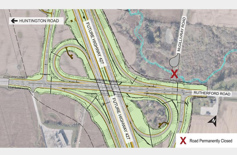
A design drawing showing the Highway 427 / Rutherford Road interchange configuration. The intersection of McGillivray Road and Rutherford Road must be closed to allow for Highway 427 construction.
