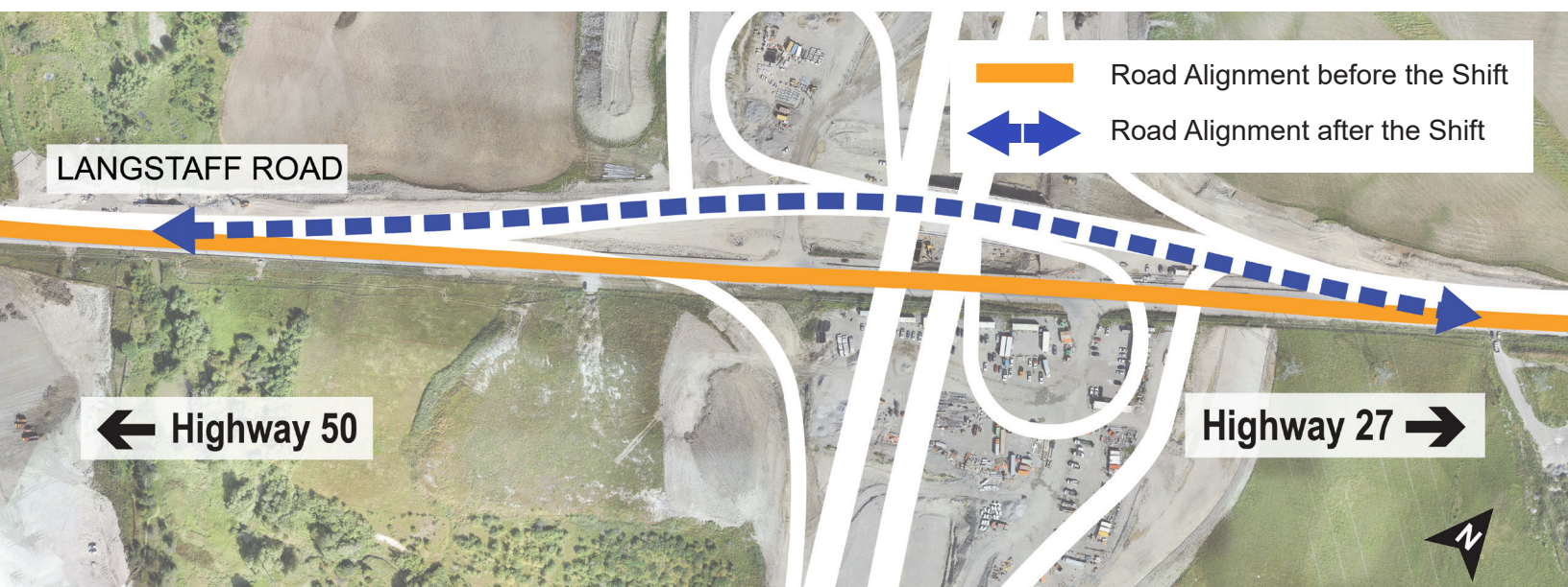
Diagram illustrating how Langstaff Road shifted at the end of 2019. Diagram not to scale.
