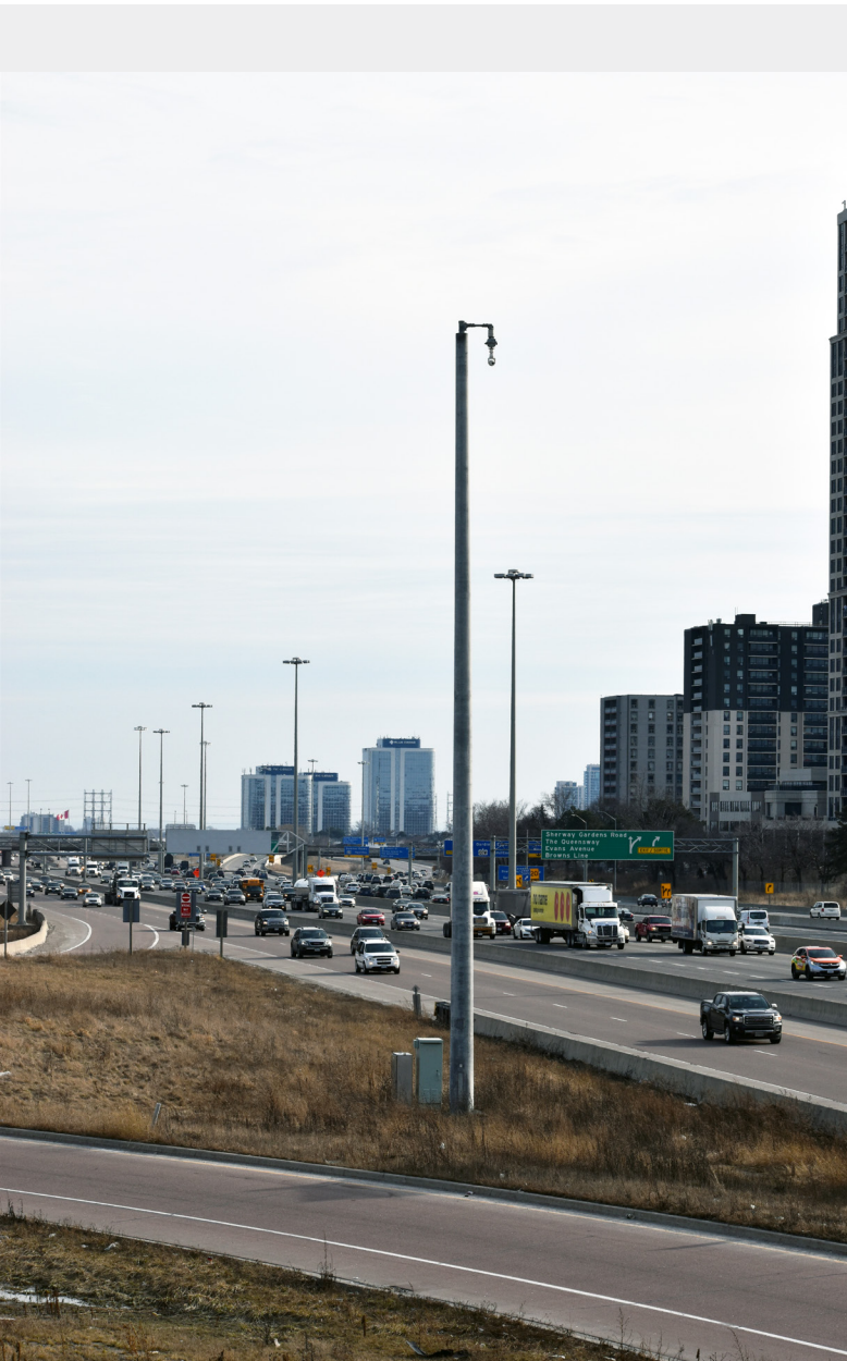
A CCTV camera mounted on a pole at the Highway 427 & Burnhamthorpe Road interchange in Toronto.
