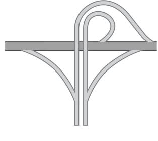
suggests, resemble the shape of a trumpet when viewed from above. They are commonly used when a highway terminates at another highway or a local arterial road perpendicularly in the shape of a "T". Motorists will find a newly built trumpet interchange on the Highway 427 Expansion at the Major Mackenzie interchange.
